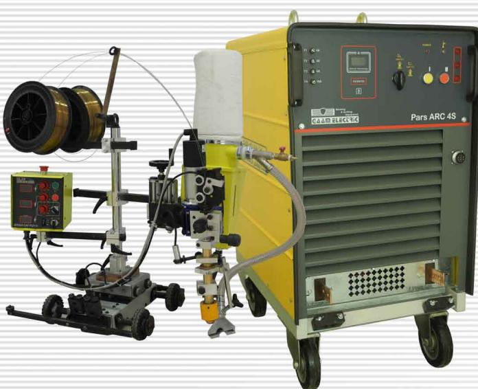
Submerged Arc welding (SAW) process can be performed in various ways, from the simplest process using a single wire to more advance Twin-Wide. Choosing the right SAW process for your operation can help you increase deposition rates and productivity.
